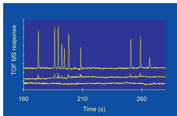
**Figure 3.** Time-scheduled reconstructed ion chromatogram using quantification masses of ten OPPs obtained after injection of 1  $\mu\text{L}$  1000-fold concentrated river Rhine water extract. Lower trace: river water blank; middle trace: same sample spiked at 0.1  $\mu\text{g/L}$ ; upper trace: spiked at 1  $\mu\text{g/L}$ . Elution order as given in table 1.
