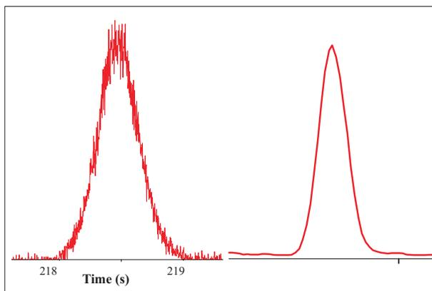
Figure 1. TIC 500 pg Diazinon at 500 and 20 Hz.
