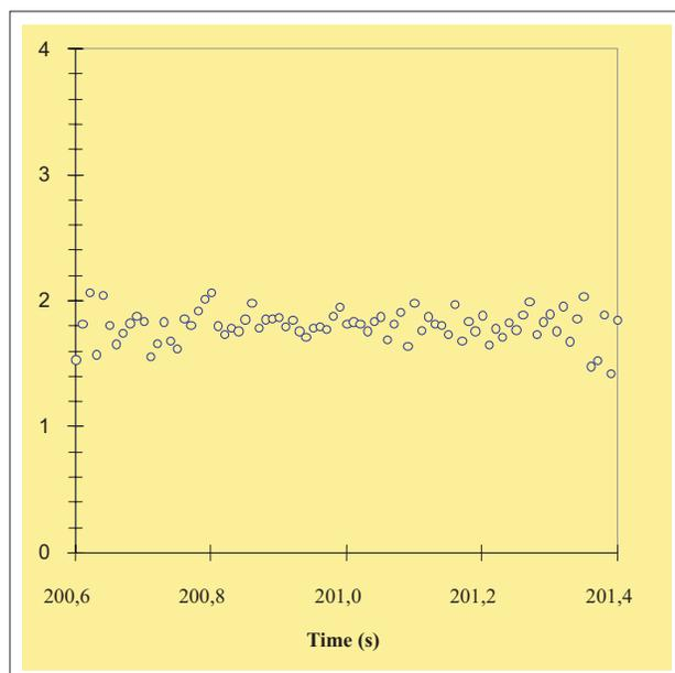
**Figure 2.** Mass ratio of  $m/z$  193 and  $m/z$  137 over the peak profile of diazinon at 100 Hz.
